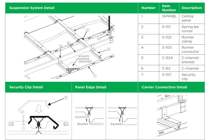
The ceiling is suspended by Spring tee runner (2) which is fixed at the bottom of the C-channel (6) and connected by the Runner clamp (3) with a distance of 600mm centre to centre.
